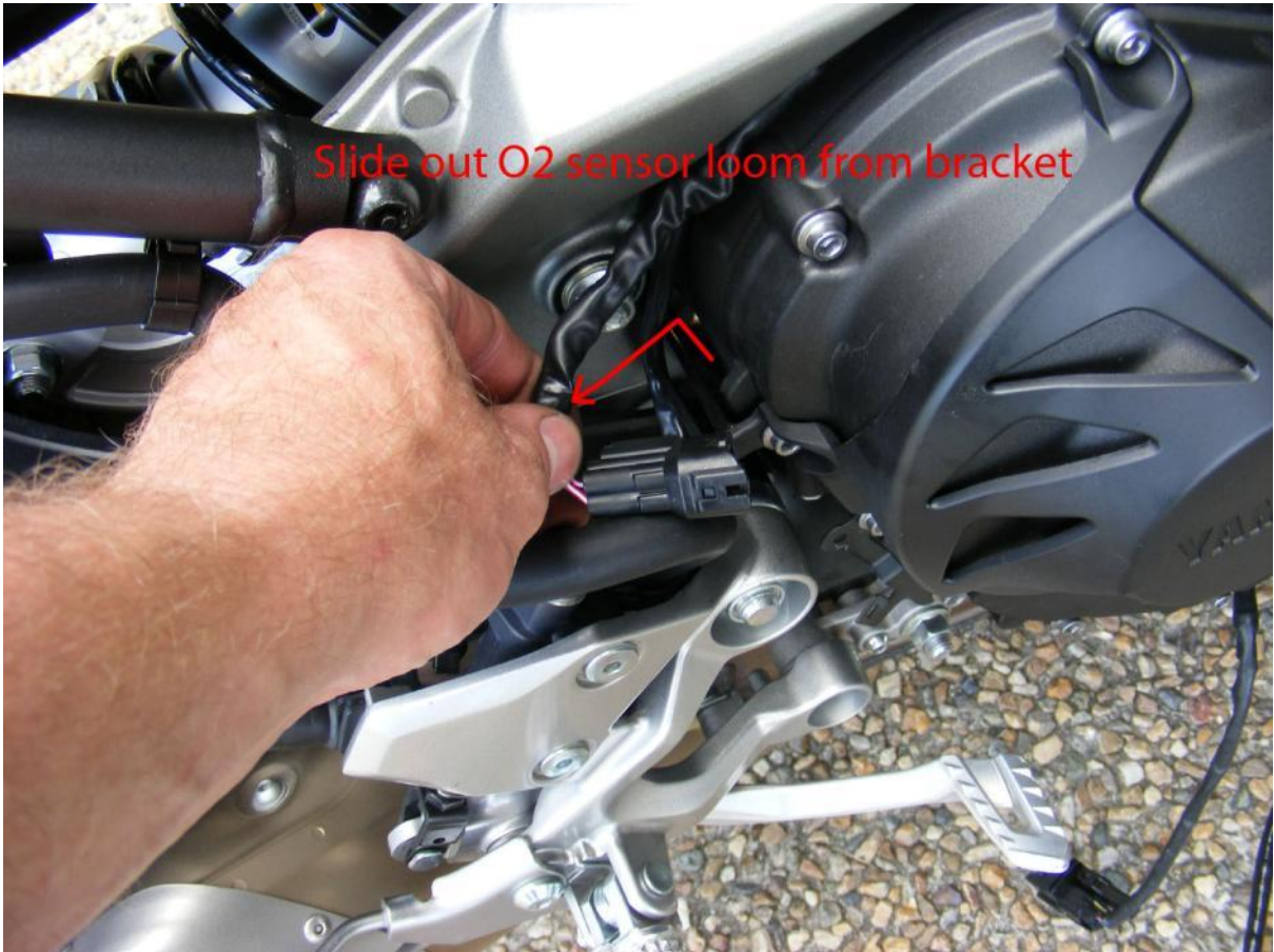
To unplug the O2 sensor Pull this tab outwards with your finger nail to release the catch, then pull the connectors apart.
